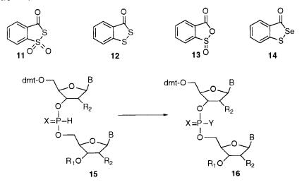
$R_1 = \text{various hydroxyl protecting}$  groups,  $R_2 = H$  or OTBDMS 15a, X=0 16a, X=0,  $Y=S^-$ ;16b, X=S,  $Y=O^-$ ; 16d, X=0,  $Y=Se^-$ 16e, X=S,  $Y=Se^-$ 16e, X=S,  $Y=Se^-$ 16e, X=S,  $Y=Se^-$ 16e, Y=S0.
